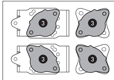
Attach the adapter (3) with your GPS mount. Tighten the screws carefully.
