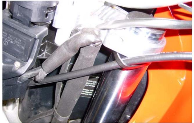
**Wiring harness (5&6):** Routed as original but not fixed with the original cable ties.
