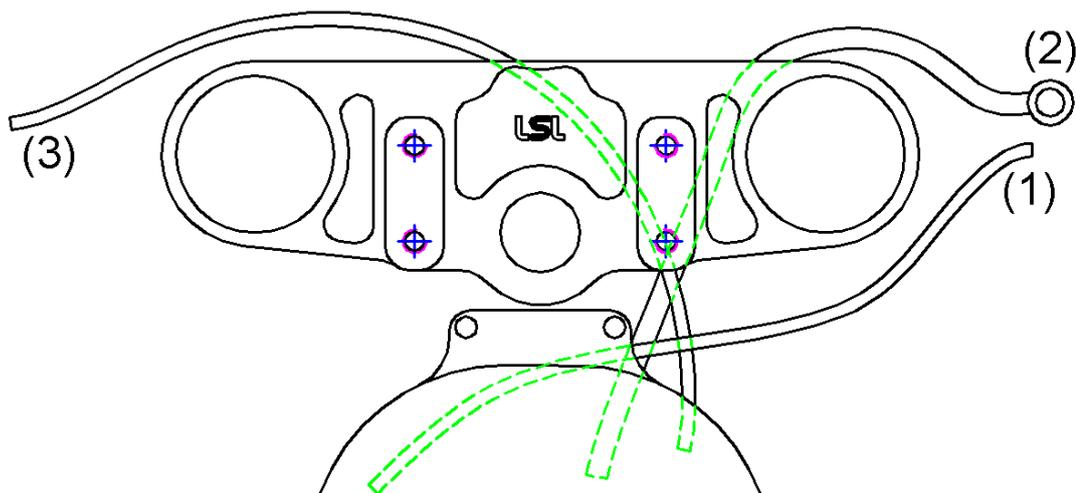
**Throttle cable (1):** To reroute the throttle cable it's necessary to loose the steering damper and the radiator. Route the cable to the right side and guide it behind the right stanchion to the control unit. Use the fastener for the clutch cable, underneath the steering head, to fix the throttle cable and the brake hose. Check throttle cable for free movement on every steering angle.
