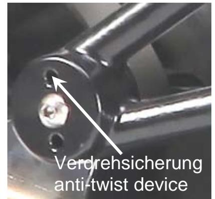
Mould one pin mirror-inverted, as shown, into each bracket. Assure that pins reach their dead stop and sit firmly. Use the upper hole on each side of the frame as anti-twist device.
